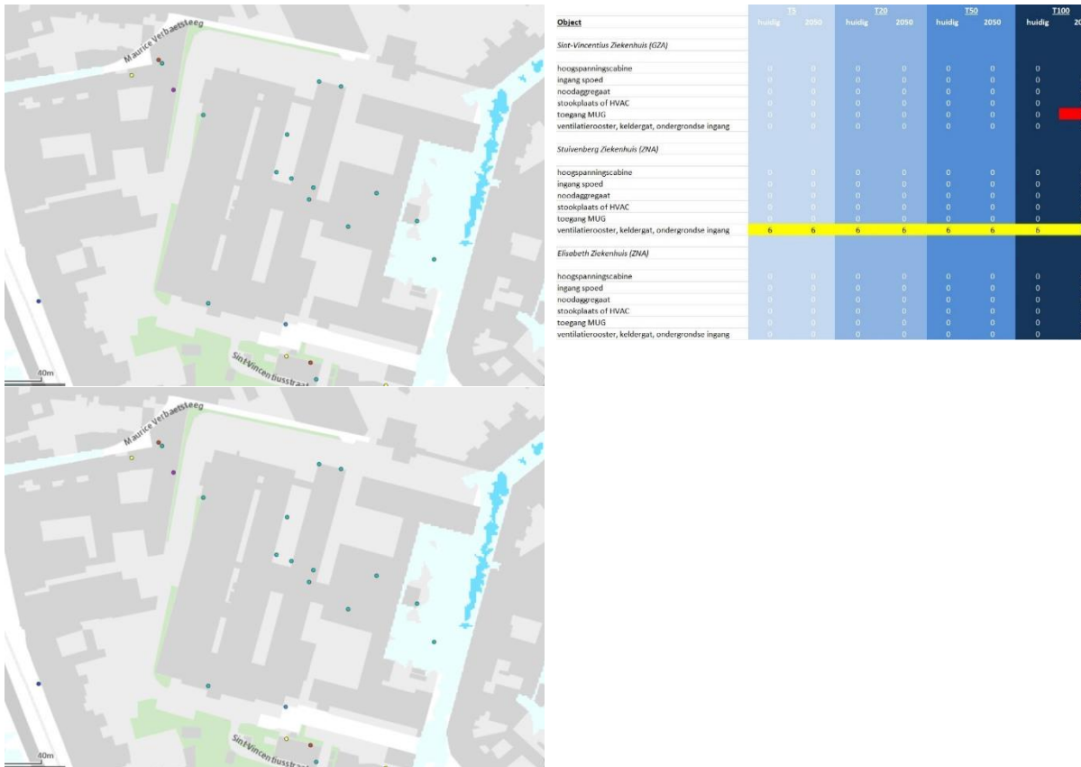
Figure 7-4 Results from the Climate-fit.city flood impact mapping of hospital infrastructure in Antwerp. Left: Vincentius Hospital Antwerp and its vulnerable locations, in relation to T100, current climate. Right: Identification of likelihood of flooding for different systems in three hospitals in the Antwerp city centre.
